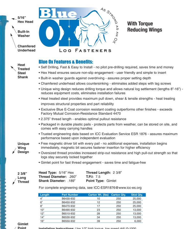
**Installation Instructions:** Use 1/2" high torque, low speed drill (0-1000 RPM) with 5/16" hex driver. Allow for minimum 2.5" penetration into the bottom log with 1/4" countersink depth. Always consult your engineer for proper placement procedures.
